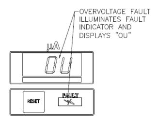
Figure 28: Over Voltage Fault Display
