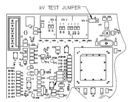
**Figure 21: Lockout Jumper Location**
