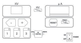
Figure 3: 9060 Operator Interface
