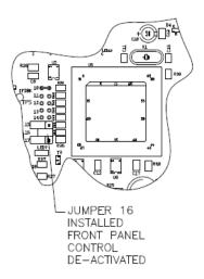
Figure 19: Jumper Location - Front Panel Lockout
