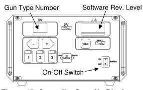
Figure 15: Controller Start-Up Display
