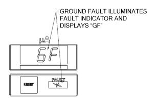
Figure 24: Ground Fault Display
