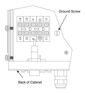
Figure 13: Ground Screw on Base Plate
