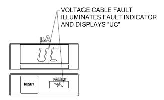
Figure 27: Voltage Cable Fault Display
