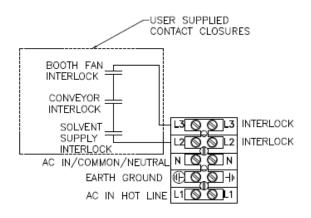
Figure 9: TB1 Interlock Wiring
