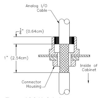
Figure 7: I/O Cable Stripping
