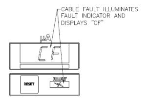
Figure 23: Cable Fault Display
