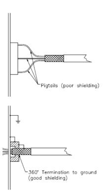
Figure 5: Pigtailing Connection
