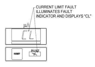
Figure 26: Current Limit Fault Display
