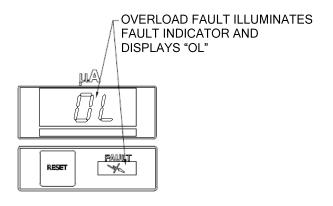
Figure 25: Overload Fault Display
