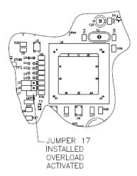
Figure 20: Jumper Location - Overload
