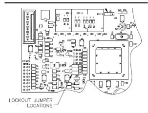
**Figure 18: Lockout Jumper Location**
