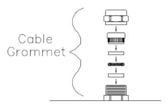
Figure 6: Cable Grommet
