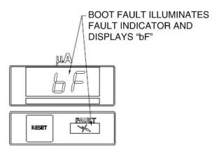
Figure 30: Boot Fault Display
