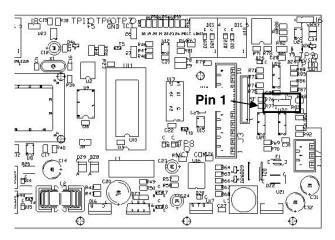
Figure 14: PC Mainboard Jumper J5 Location
