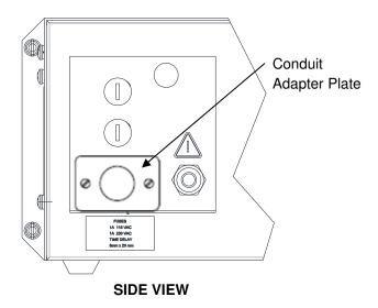
Figure 10: Installation of Conduit Adapter Plate
