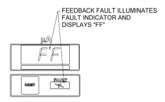
Figure 29: Feedback Fault Display
