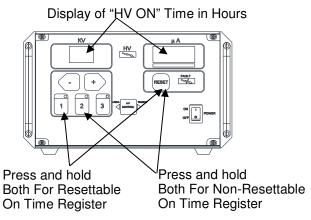
Figure 17: Display "High Voltage On"
